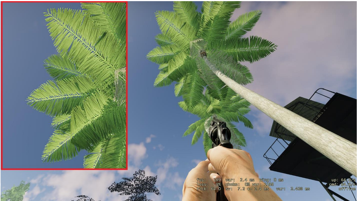
Figure 12: MSAA 8x, SMAA disabled, jagged edges can be seen on palm leaves
