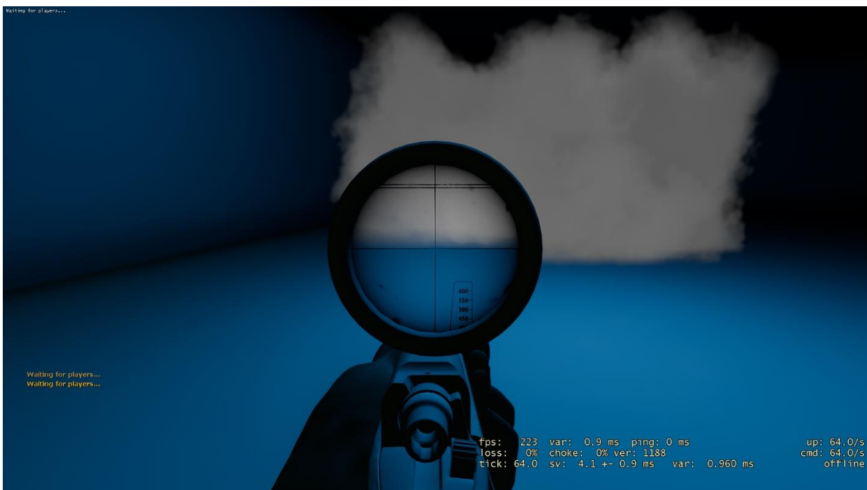
Figure 48: Soft particle appears correctly in Sniper RT camera without any extra depth buffers and render passes
