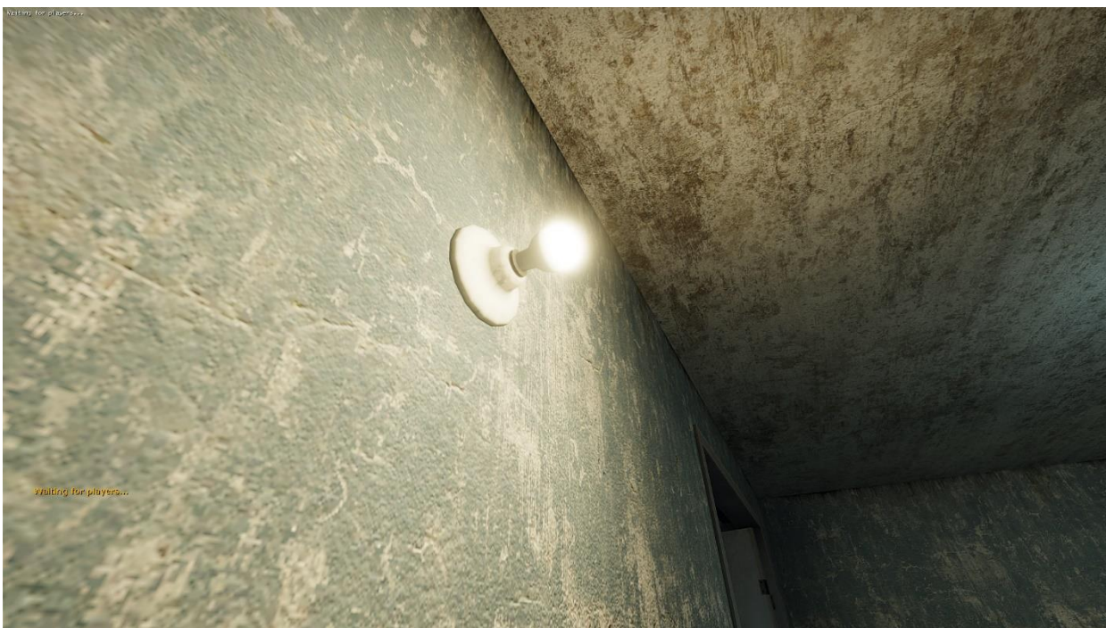
Figure 5: This is the result of Floating Point HDR + New Bloom working together. Pixels with high luminosity values make bloom contribute to final image, while the rest of the scene remained as-is. In the end – lamp glows by itself, no need to use “glow” sprites anymore.
