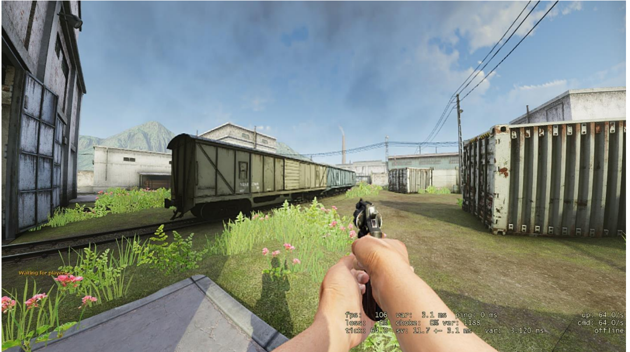
Figure 58: Example scene with FOV 150 and barrel distortion applied to neutralize FOV artifacts.
