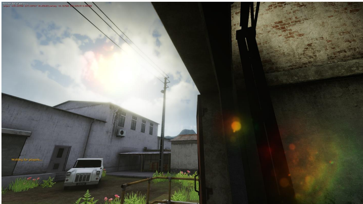
Figure 3: Floating Point HDR – More color variations, bloom is now taken in account and makes bright areas stand out and glow. As well other effects like Lens Flare can now utilize HDR bloom buffer to detect bright pixels and generate flares from them. MSAA quality difference is negligible.
